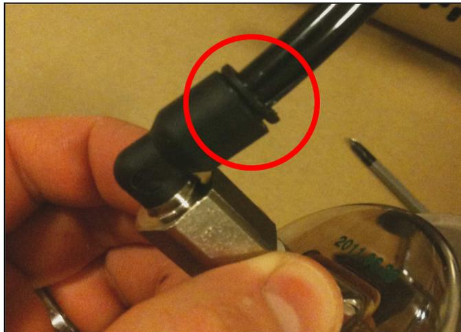
**Figure 6** Pressure Gauge Tubing Removal
